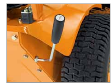
Bottom: Pneumatic tyre for stable ground contact on uneven surfaces.
