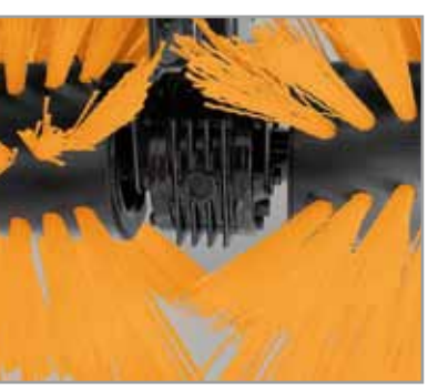
Top: Adjustable working angle with a single lever. Bottom: Centrally driven brush to allow brushing to the edge of either side
