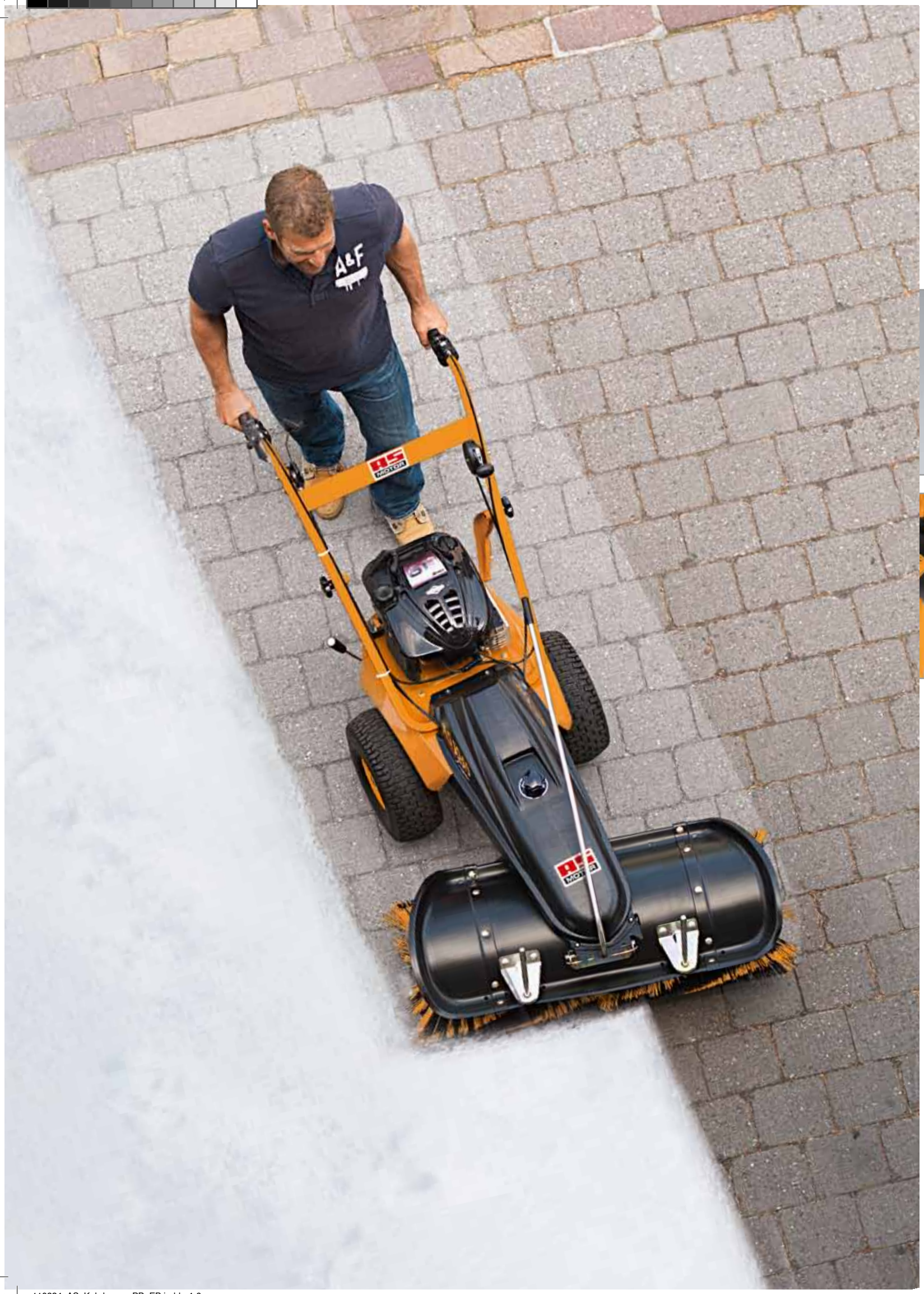
Top: Adjustable working angle with a single lever. Bottom: Centrally driven brush to allow brushing to the edge of either side
