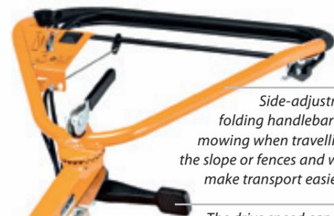
Side-adjustment and folding handlebar facilitate mowing when travelling along the slope or fences and walls, and make transport easier as well.
