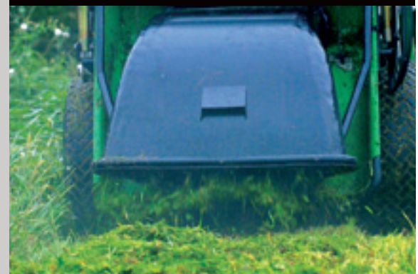
tall grass cutting with hydraulically controlled deflector
