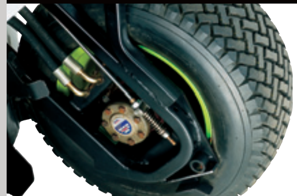
no rear axle, hydraulic wheel motors
